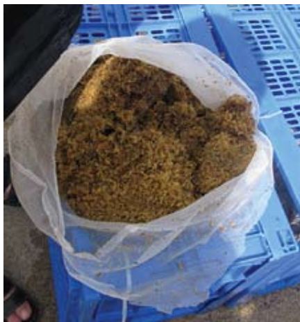
Wet sphagnum moss pulled from the surge tank for the Olympic-sized pool. The moss significantly reduced chlorine loads, pool maintenance and impacts to swimmer’s eyes, skin, hair and swimsuits. (Photo credit: Laurel Edwards, City of Saint Paul Parks and Recreation)
