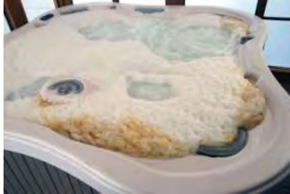
Even a brand new spa can exhibit biofilm buildup (foam and brown area appear during flushing process)
